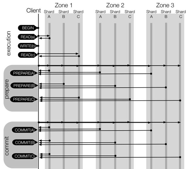
Figure 6: Example read-write transaction in TAPIR. TAPIR executes the same transaction pictured in Figure 2 with less redundant coordination. Reads go to the closest replica and `Prepare` takes a single round-trip to all replicas in all shards.
