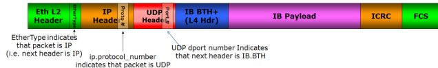
Figure 1: Structure of a RoCEv2 (RDMA over Converged Ethernet) packet, from the spec [22]. These packets operate over IP and UDP, so RDMA must provide reliability and ordering semantics. Nothing is encrypted or authenticated.
